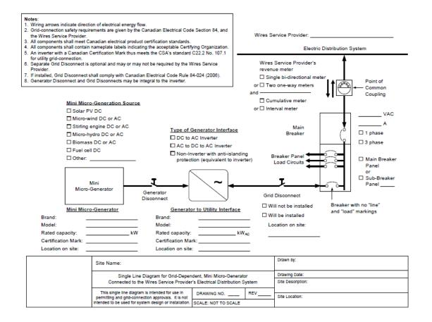
*Note – 2018 CE Code 64-218 (5) also requires the location the device to initiate rapid shut down to be shown on the Single Line Diagram*
